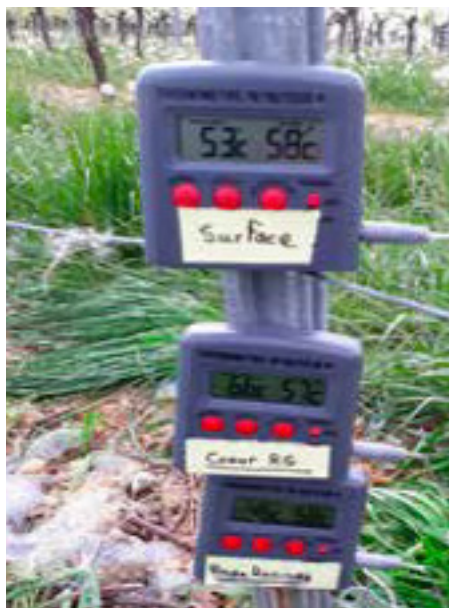
The three thermometers measured the temperature of the foam.
